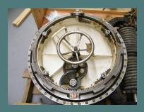
Dry deck shelter hatch. Lubrication is needed on all internal gears and locking ring threads.
