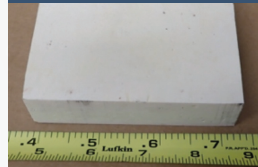
Figure 1. ThermaSilence Sound Damping Material that meets MIL-STD-2031 “Fire and Toxicity Test Methods and Qualification Procedure for Composite Materials Used In Hull, Machinery, and Structural Applications Inside Naval Submarines”
