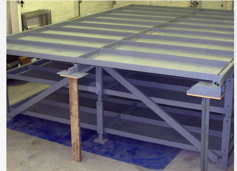
TRI Austin's ThermaSafe composite reconfigurable berth for the Virginia-class submarine torpedo room. This unit has been delivered to NAVSEA and passed a full-room fire test at NSWCCD.
